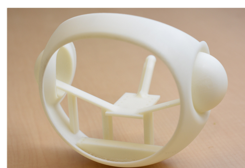
Isometric view of Lil'Flo shell, showing internals
