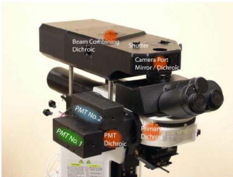
Prairie Technologies Ultima Two-photon Microscope with Olympus BX61WI motorized upright microscope.
