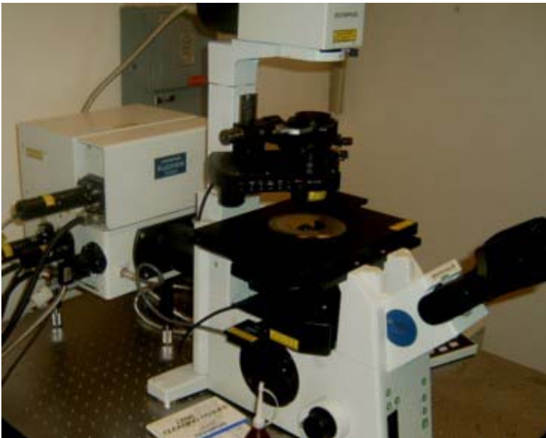
Fluoview FV1000 unit with IX81 motorized inverted microscope
