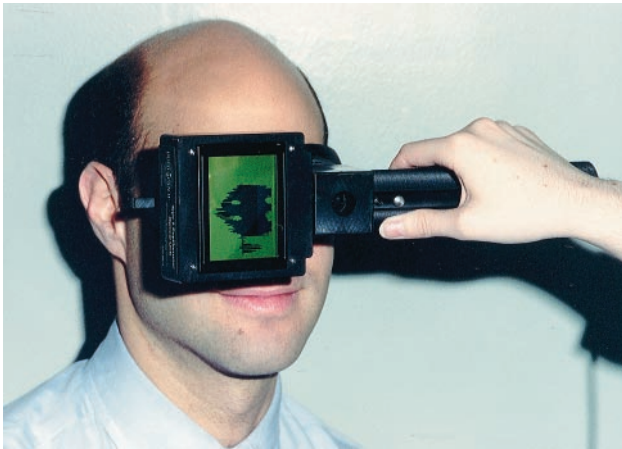
Figure 1. Pupilscan pupillometer during testing. The instrument is lightweight and approximately the size of a flashlight. A real-time pupillary image is seen during testing on the liquid crystal diode (LCD) display as well as on the computer screen. The patient maintains distance fixation in a dimly lit room through the hole in one of the eyepieces (left eye in this photograph). The instrument simply can be flipped to record from the other eye if desired.
