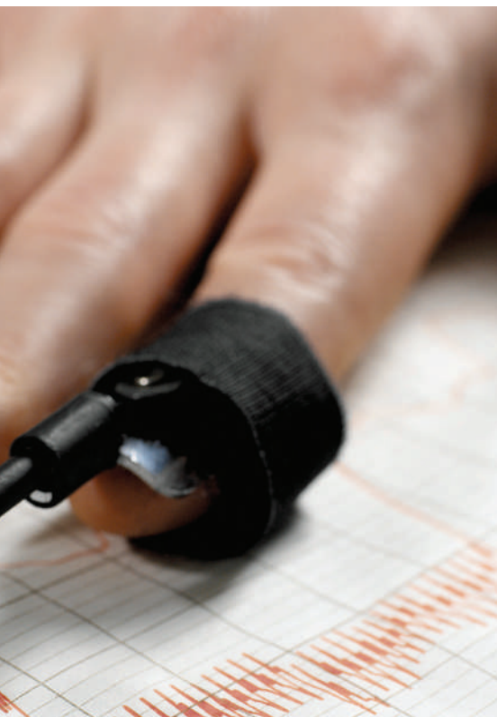
Caught out: lie detectors that use MRI scans (left) capture brains in the act of deception, whereas conventional methods rely on stress-induced changes such as fluctuating pulse rates (above).
