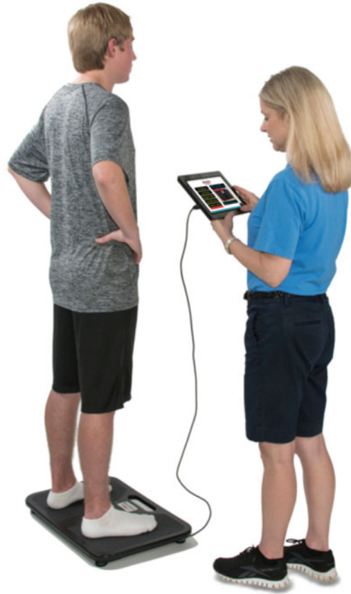
Fig. 2 The BTrackS portable force plate system. Image used with permission from [150]
