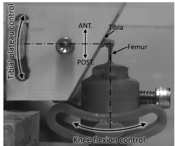
**Figure 2:** Instron setup to quantify the stability of murine knee. The custom fixtures allow for fine adjustment of knee flexion and orientation of the tibial plateau.
