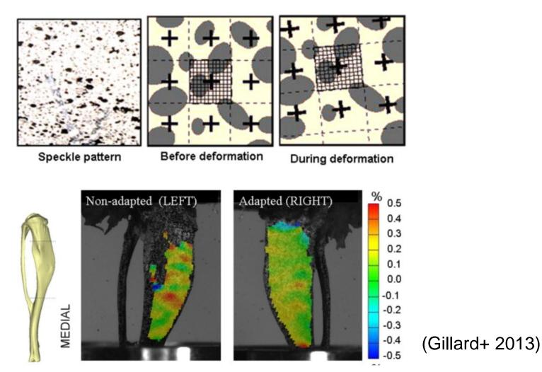
• DIC traces the deformation on the specimens surface.
