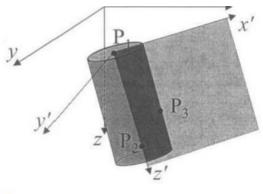
P1: the coordinates of the new origin P2: the coordinates of a point on the new Z-axis
