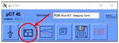
(Optional) If the scanner hasn't been used for the last 8 hours, you will see the "Information" window, and wait for the X-ray tube to warm up (15~20 min).
