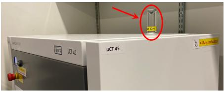
(2) The Door Locker indicator shows unlocked
