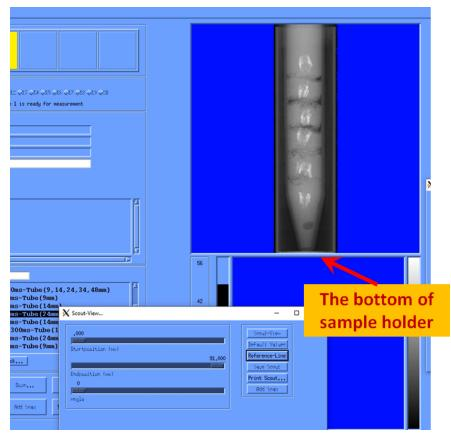
Click the "Reference-Line" in the "Scout-View..." window, hover the mouse to your desired region. If necessary, press and hold the Shift key to adjust the scan slice number. Once you have identified your region of interest, click the Left button of the mouse to set your reference line.
