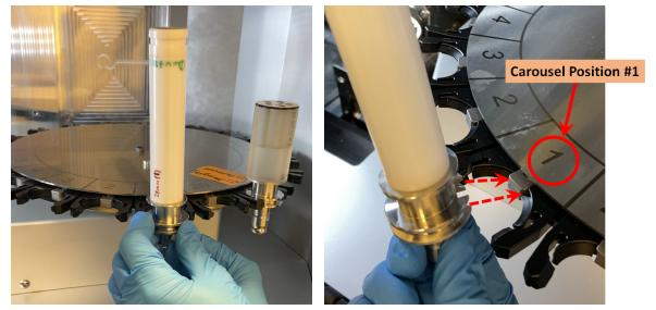
**IMPORTANT:** Make sure the sample holder is loaded CORRECTLY onto the carousel!
