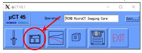
2. (Optional) If the scanner hasn't been used for the last 8 hours, you will see the "Information" window, and wait for the X-ray tube to warm up (15~20 min).
