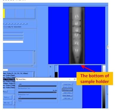
3. Click the "Reference-Line" in the "Scout-View..." window, hover the mouse to your desired region. If necessary, press and hold the Shift key to adjust the scan slice number. Once you have identified your region of interest, click the Left button of the mouse to set your reference line.
