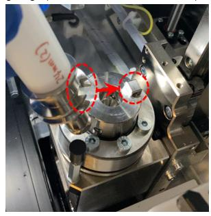
IMPORTANT: Make sure the sample holder is loaded fully on the rotation/loading stage!
