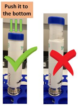
2. Before proceeding to the next step, please <u>use a paper towel to wipe any liquid outside the sample holder. Any liquid outside the holder can damage the scanner!</u>
