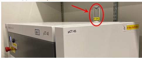
(2) The Door Locker indicator shows unlocked
