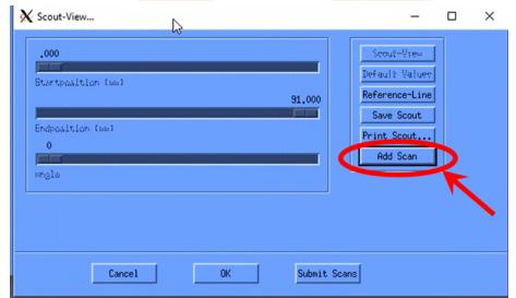
How to set up a scan on µCT45 (Non-carousel version)
