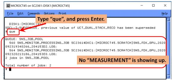
Note: If no "<u>MEASUREMENT</u>" is showing up after the "que" command, but the <u>Door Locker indicator</u> still show <u>locked</u>, please click the "<u>Scan</u>" button in the control box (shown below) to unlock.
