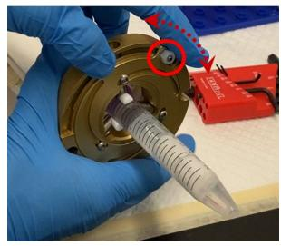
Note: If the screw is too tight to adjust, use an allen wrench to loosen the 3 screws in the inner circle.
