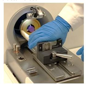
3. Lock the secure handle on the animal bed to the scanner track, and then close the hood.
