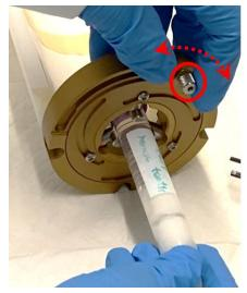
Note: If the screw is too tight to adjust, use an allen wrench to loosen the 3 screws in the inner circle.
