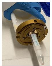
2. Loosen or adjust the screw accordingly to ensure your tube fits securely in the tube holder.
