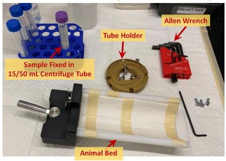
Align the 3 holes in the tube holder to the 3 threaded holes in the animal bed. Using an allen wrench, fixate the 3 screws to secure the tube holder to the animal bed.
