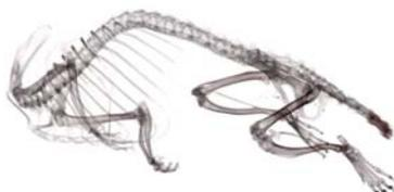
Micro-CT scan at 28  $\mu\text{m}$  isotropic resolution of a transgenic mouse presenting a Paget's disease-like phenotype with osteopenia of femoral trabeculae, visualized by red glass volume rendering. (J.P. Taylor, et al.)
