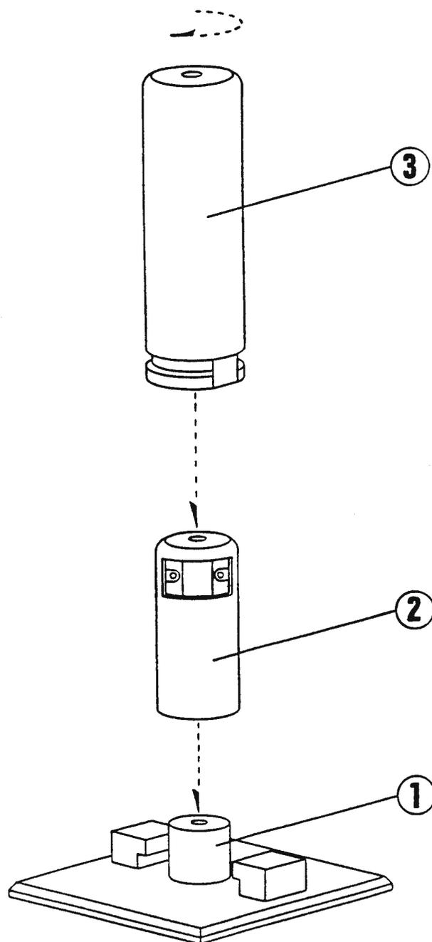
**FIGURE 1** Schematic diagram for setting up the Push Column Beta Shield Device. (1) Beta shield base; (2) column beta shield with the column-locking mechanism; (3) syringe cover.
