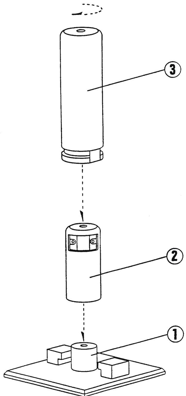
**FIGURE 1** Schematic diagram for setting up the Push Column Beta Shield Device. (1) Beta shield base; (2) column beta shield with the column-locking mechanism; (3) syringe cover.
