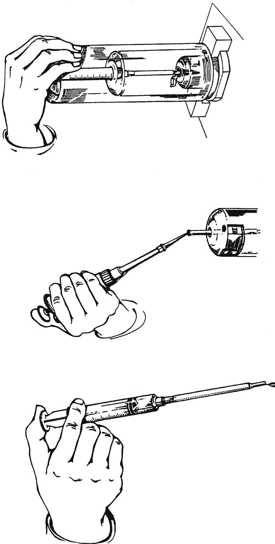
**FIGURE 2** Schematic diagram for preparing the columns and for loading and separating the sample using the NucTrap probe purification columns and Push Column Beta Shield Device. (A) Prewetting the column. (B) Loading the sample onto the resin at the top of the column. (C) Pushing the sample through the column.
