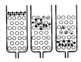
solutes will enter the gel matrix and are retained on the column longer. The retention time is inversely proportional to the size of the solute.
