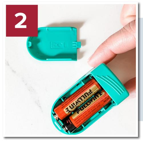
Unpackage the two AAA batteries that came with the device and install them.
