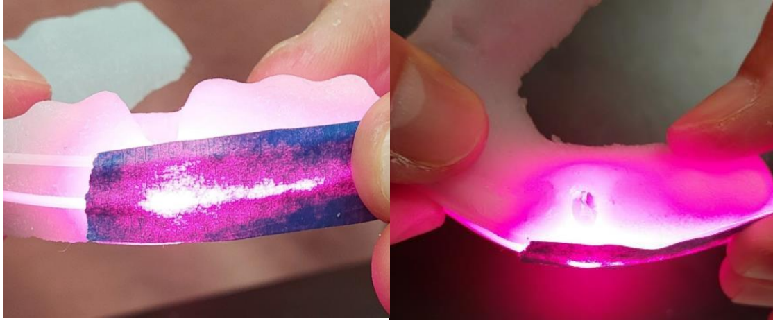
Figure 29. Semi-infinite device placed on 3-Dimensional phantom simulating human maxilla with extraction socket. a) lateral view. b) superior view showing that semi-infinite device is fully in contact with target surface.
