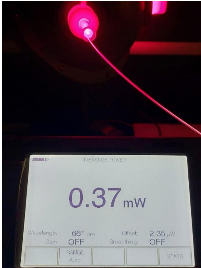
Figure 149. Bone Tissue Optical Properties. Power measurements of 661nm isotropic light source inside of integrating sphere.
