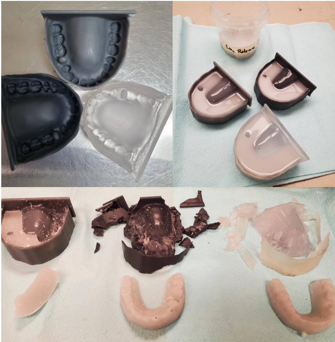
Figure 9. 3D Dental Model. a) top is traditional grey resin, left is "Flexible", right is "Elastic", b) Silicon material poured in all 3 resin materials, c) removal of phantom molds from each model (L-R traditional resin, flexible, and elastic).
