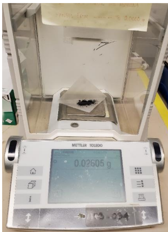
Figure 2. Measurement of Carbon to mimic human tissue optical properties of absorption.
