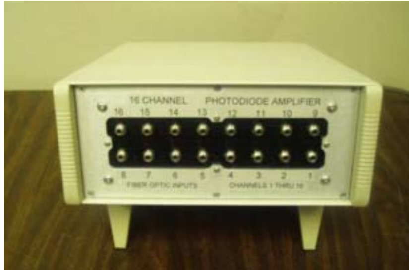
Figure 4.29: In-house built dosimetry system to measure fluence
